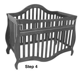
**Step 4:** Repeat Step 3 to attach the front assembly to the End Frames. Make sure that the gate folds to the outside of the crib. With the front dropped to the bottom of the bolt holes you can now tighten the bolts. Make sure that the gate locks properly in the latched position.
