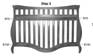
**Step 2:** To attach the Front Posts to the Front Frame you will need the other two 100mm Bolts and the other two 70mm Bolts. You will need to attach the Front Posts to the Front Frame with gate.
