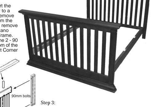
You will now attach the two short posts to the Front Frame with 4 - 90 mm bolts. Then you will need to attach the bottom base molding to the bottom of the short posts with 2 - 90 mm bolts. Then attach the Top Front Crown Cap to the Front Frame with 3 - 8 x 40 mm wooden dowels, turn the Footboard upside down and screw in 5 - 3" screws through the Front Frame into the Top Front Crown Cap. Now your Footboard is complete.
